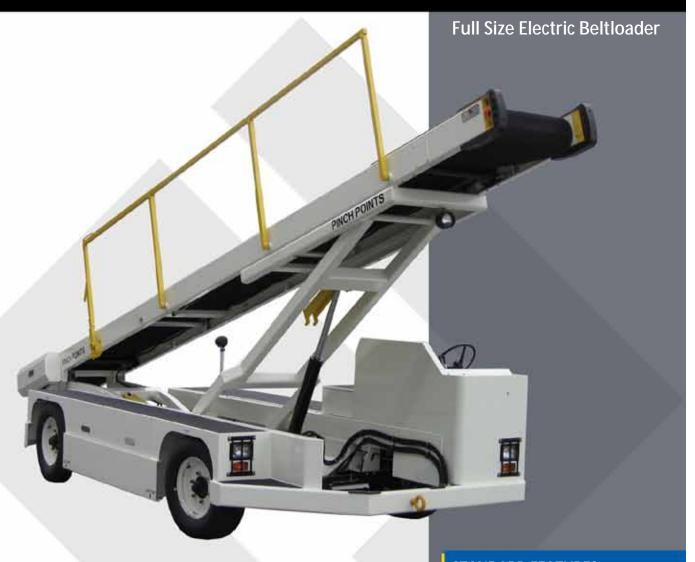
Charlatte Beltloader Model CBL2000E is capable of servicing all types of aircraft with door sill heights ranging from 30" up to 170". Power for the main drive is supplied by a 40 hp AC motor which gives the unit a 16 MPH running speed on level ground. The majority of major components are compatible with the T-137 electric baggage tractor.
